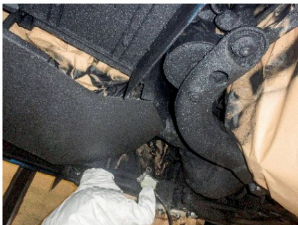
Application on a train underbody
