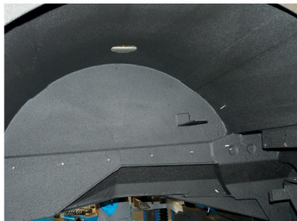
Wheel arch with Sikagard®-6682 applied
