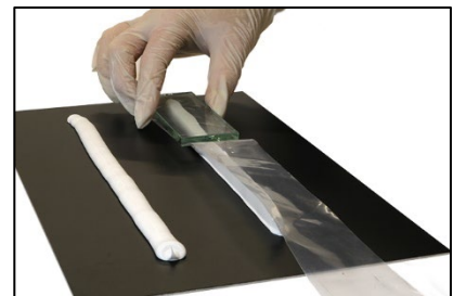
Figure 13 Press the bead to half the height
