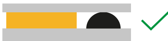
Figure 10 Positioned outside the bond line
