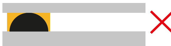
Figure 8 Spacer size too big for bond line width
