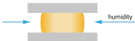
Figure 1 Humidity curing principle
